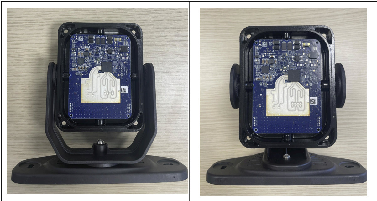
Figure 1: front view without cover with 2-axis rotating stirrup (on the left) and 3-axis rotation stirrup (on the right)
