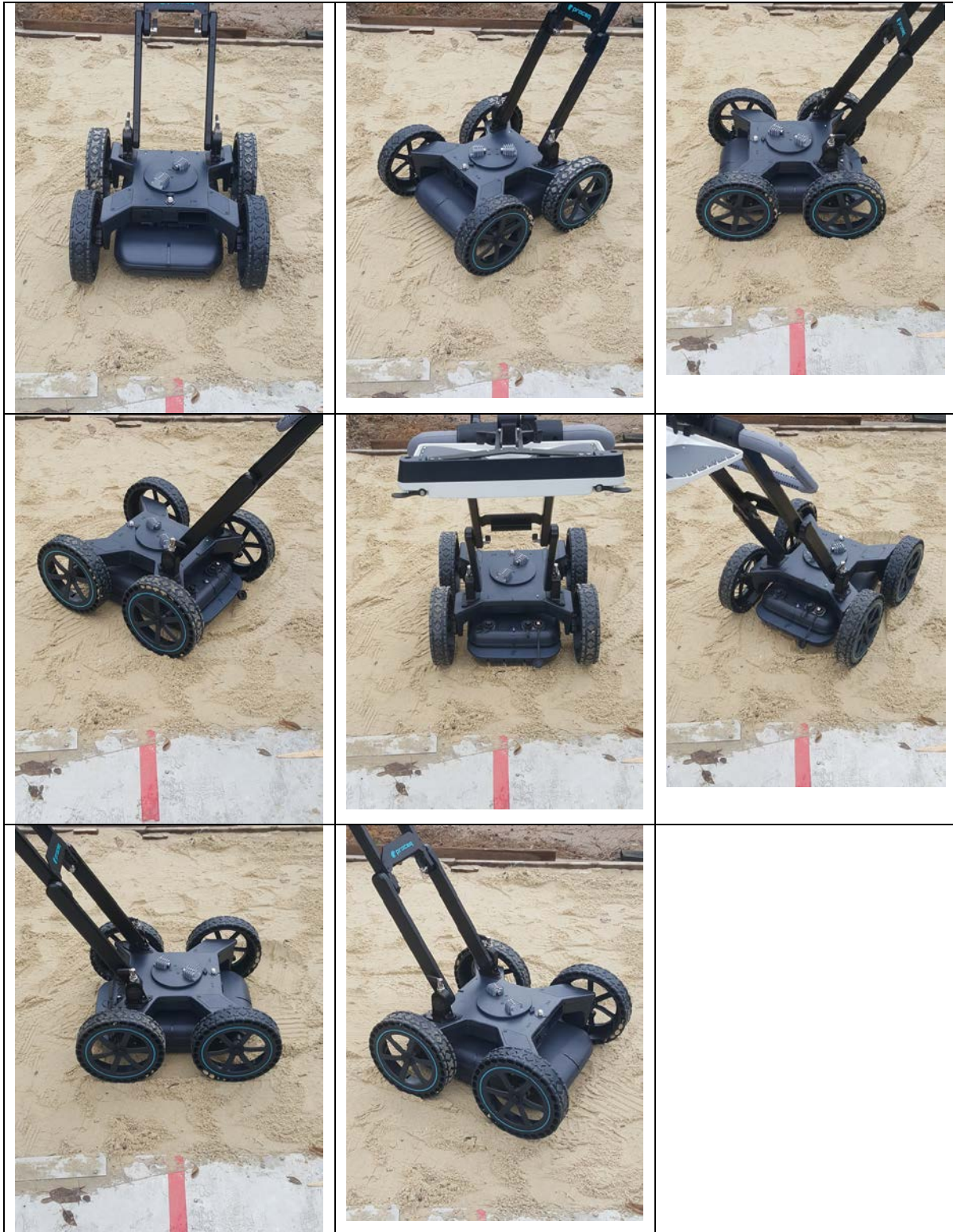
EUT Positions with 45 Degree Interval
