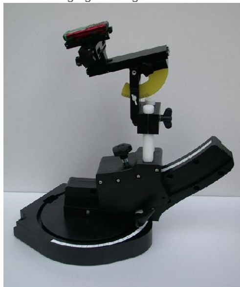
Device holder supplied by SPEAG
