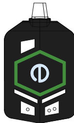
Fit Test: PASS indicator lights for a successful Earpiece Fit Test
