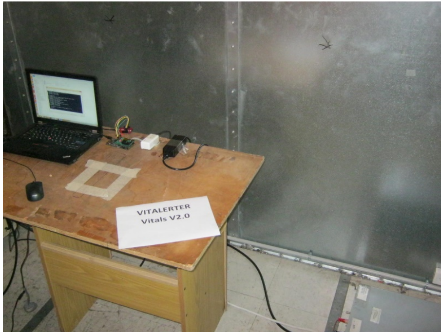
Conducted Emission from AC Mains Test
