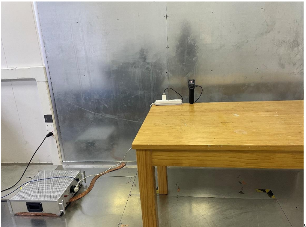
AC power-line conducted emission Test Setup
