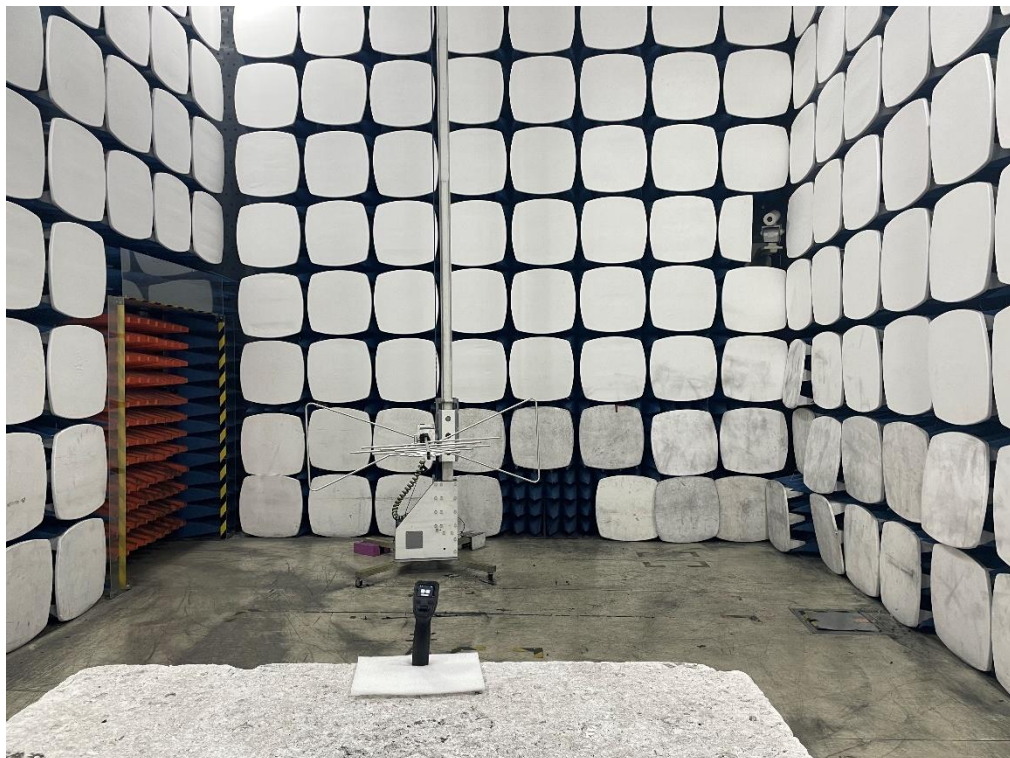
FCC Radiated Emission Test Setup-below 1GHz
