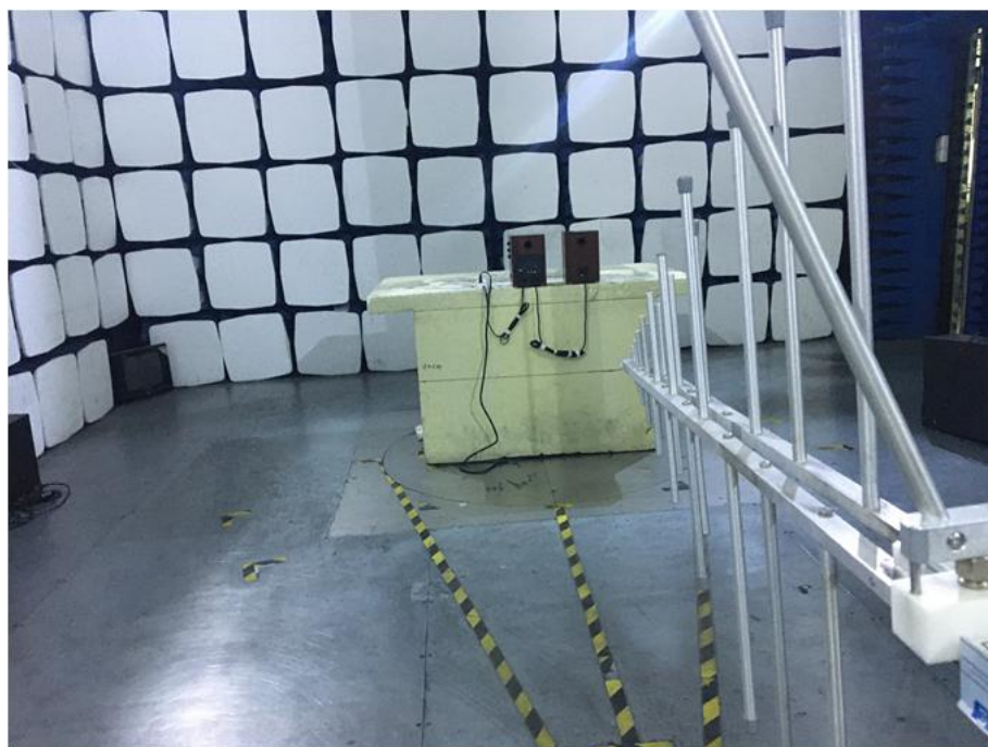
Radiation Emission Test Setup (30MHz to 1GHz)
