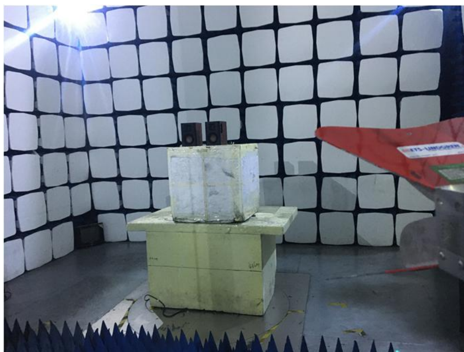
Radiation Emission Test Setup (1GHz to 18GHz)
