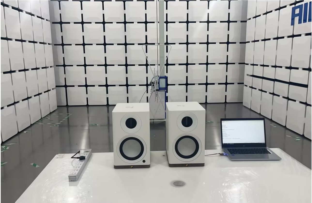
Radiated Spurious Emission Test View 1
