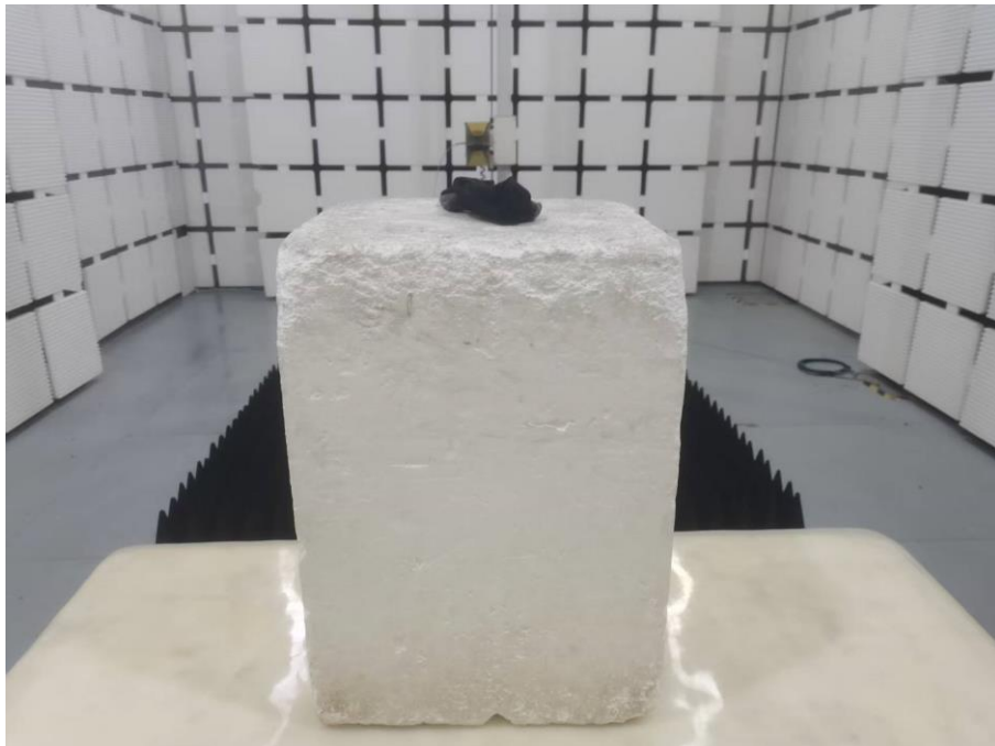
Set-up for Radiated Spurious Emission, Above 1GHz
