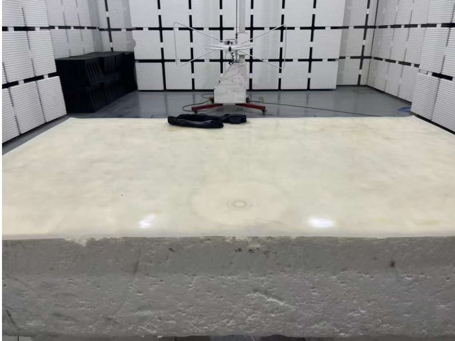
Set-up for Radiated Spurious Emission, Above 1GHz
