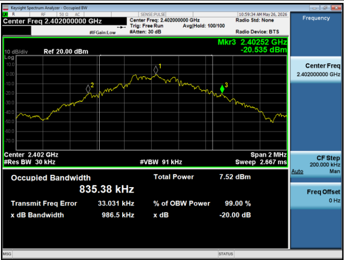
-20dB Bandwidth NVNT 1-DH5 2402MHz Ant1
