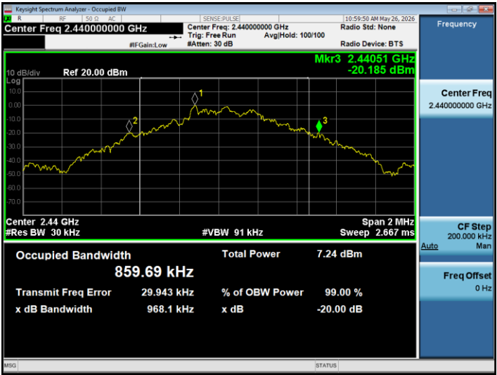
-20dB Bandwidth NVNT 1-DH5 2440MHz Ant1
