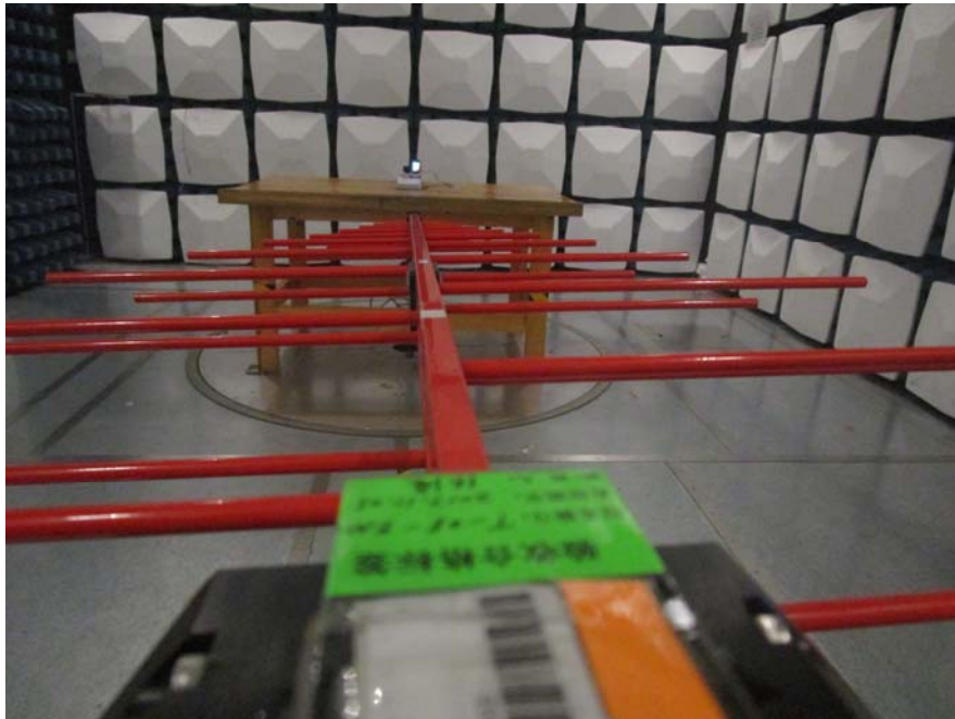
Radiated Emission View (Below 1GHz)
