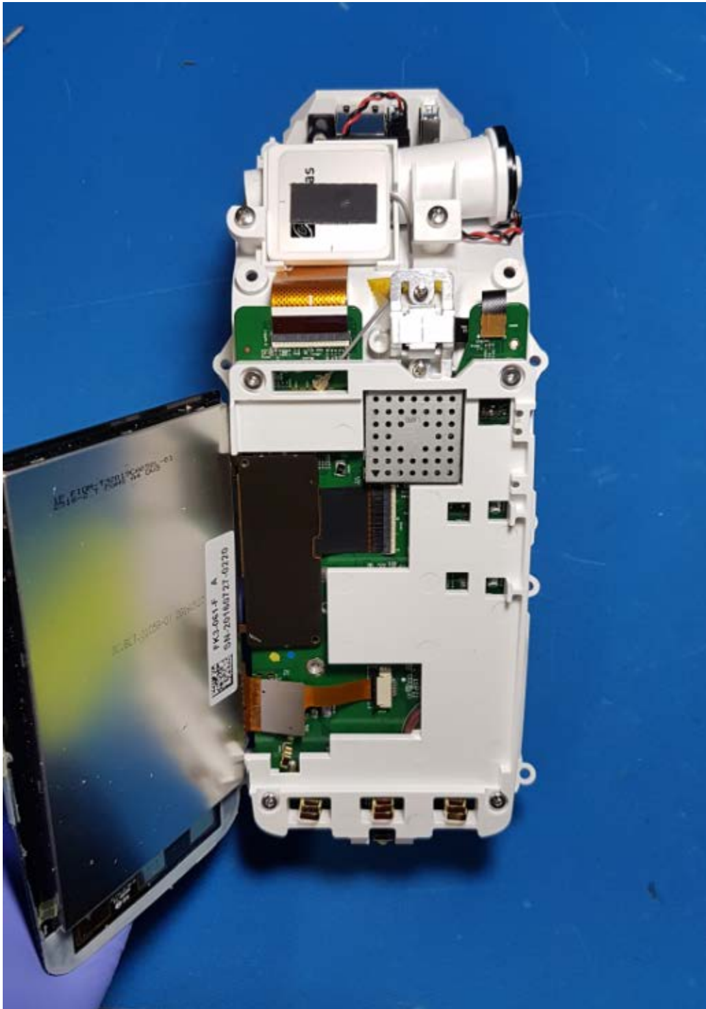
Top Side View with LCD lifted and LCD frame shown installed
