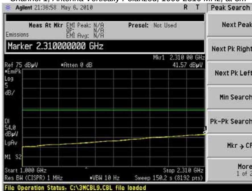
Channel 1, Antenna Vertically Polarized, 1000-2310 MHz, at 3m
