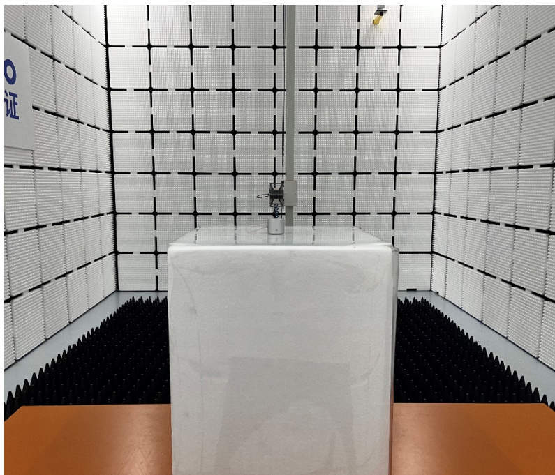
Radiated Emission Above 1GHz
