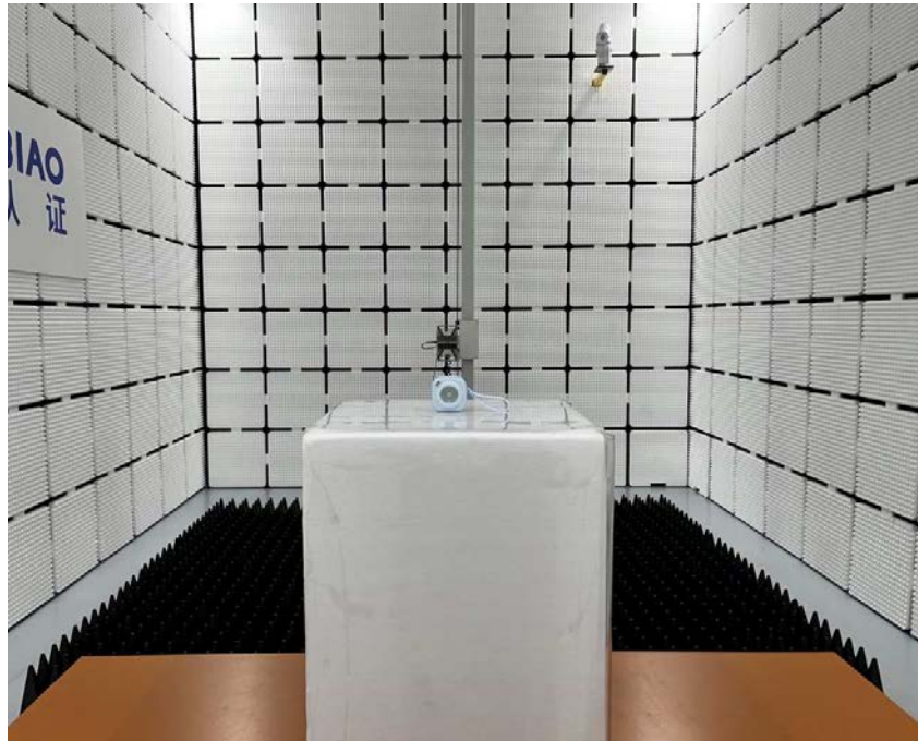
Radiated Emission Above 1GHz
