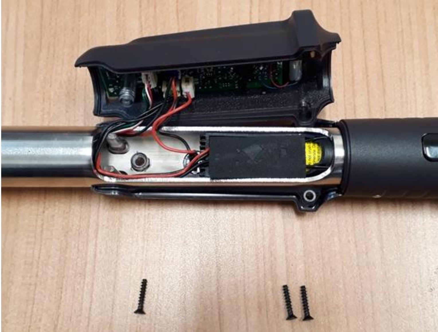
SMART TORQUE – Picture 2: USER INTERFACE DISASSEMBLED
