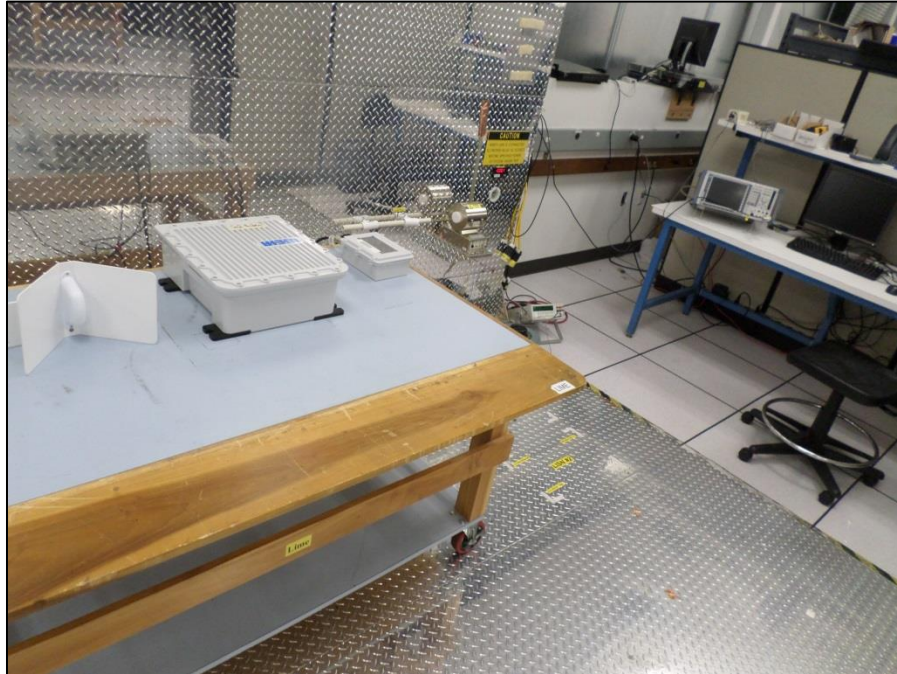
Photograph 1. Conducted Emissions, 15.207(a), CEV Station Setup
