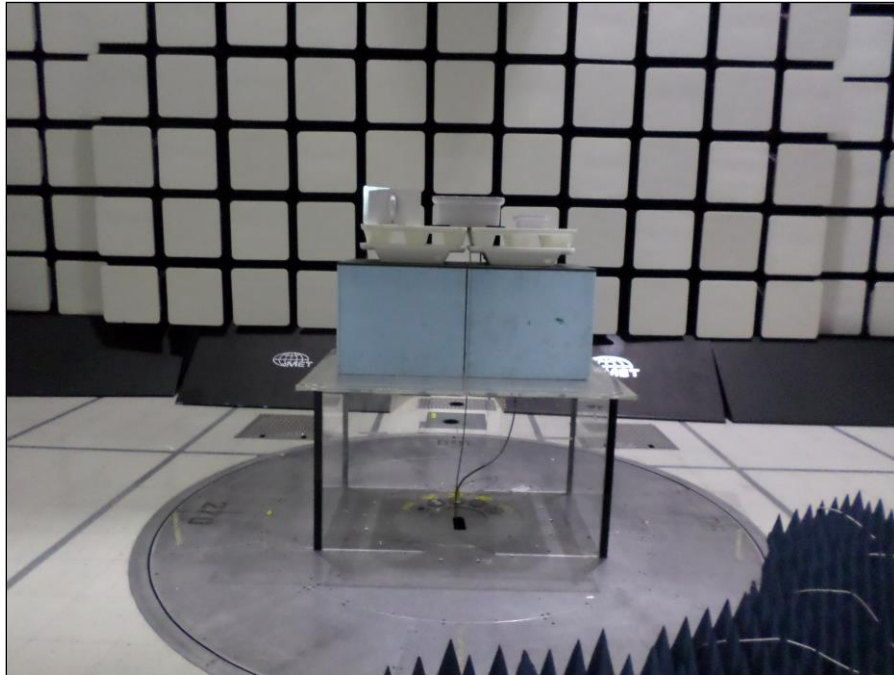
Photograph 5. Radiated Spurious Emissions, 12 dBi, 1 – 18 GHz, Test Setup, Front
