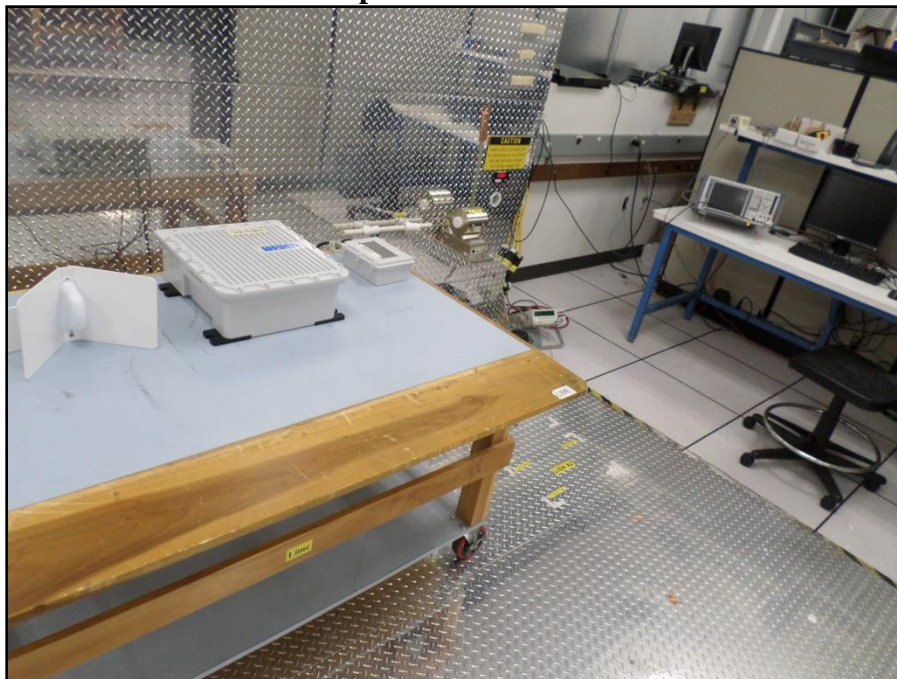
Photograph 3. Conducted Emissions, 15.207(a), CEV Station Setup
