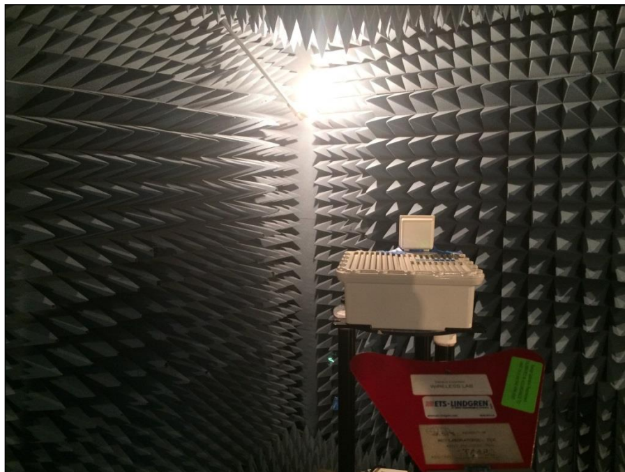
Photograph 2. Radiated Emissions, Above 1 GHz, Test Setup
