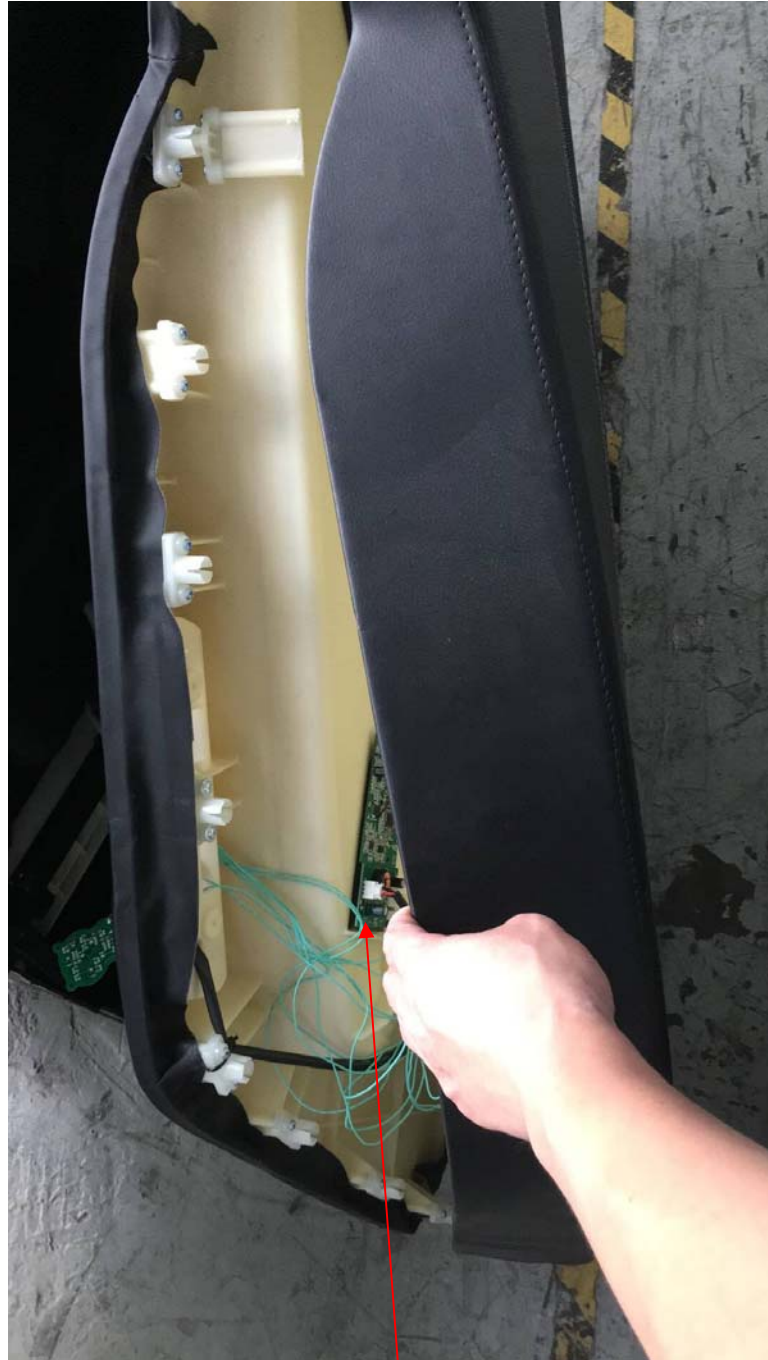
The location of the Bluetooth board
