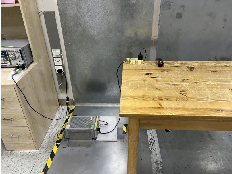
Radiated Spurious Emissions Test Frequency From 30MHz-1GHz
