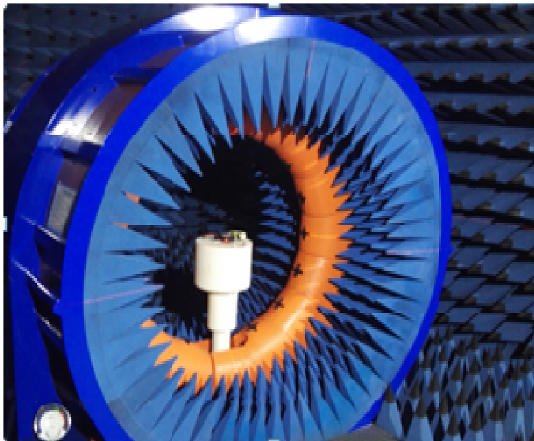
16-probe OTA testing system
