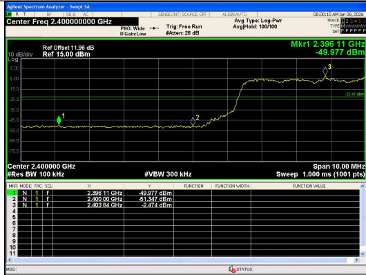
Out Of Band Emission(Left) \pi/4 DQPSK_2-DH5_Channel Hopping
