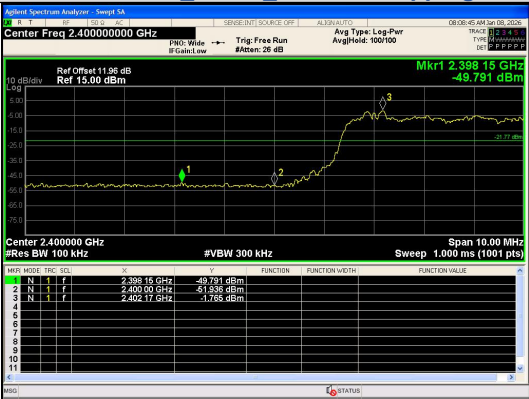
Out Of Band Emission(Left) \pi/4 DQPSK_2-DH5_Channel Hopping
