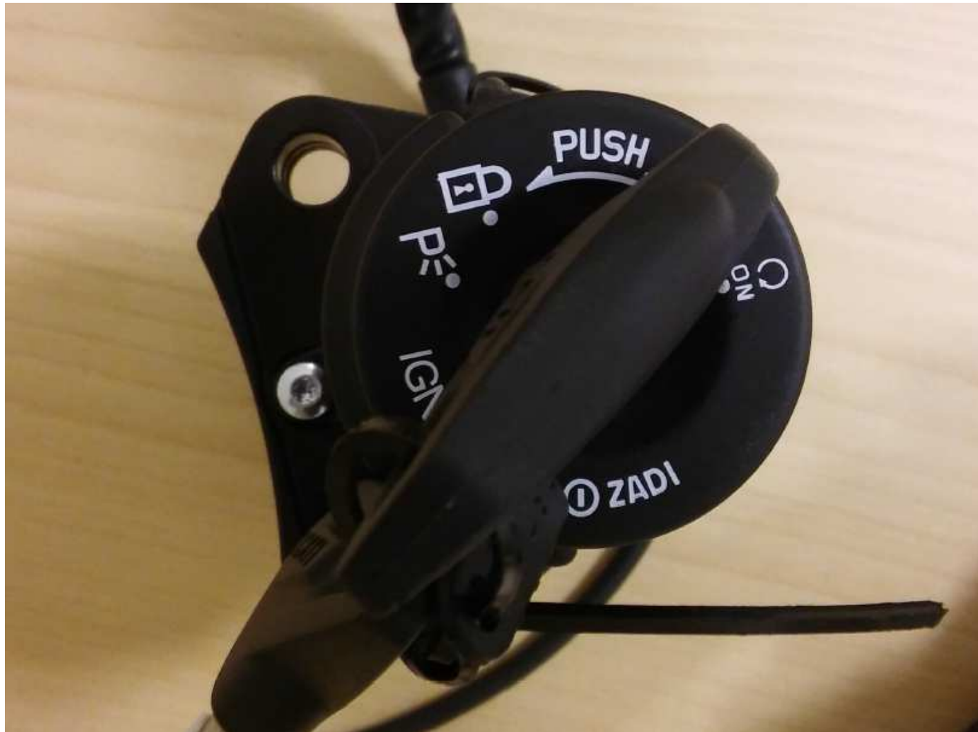
Ignition switch containing antenna (upper view)
