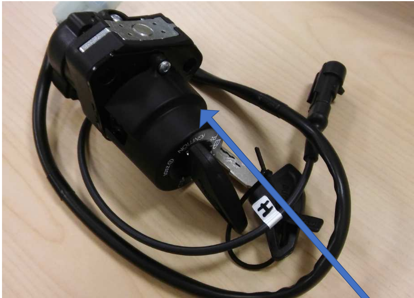
Ignition switch containing antenna (and position of antenna)
