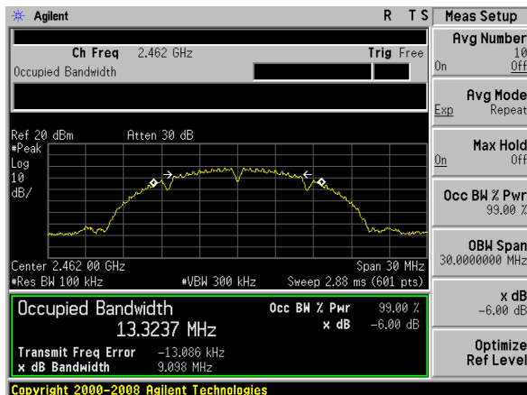
(802.11b) 6dB Bandwidth plot on channel 11
