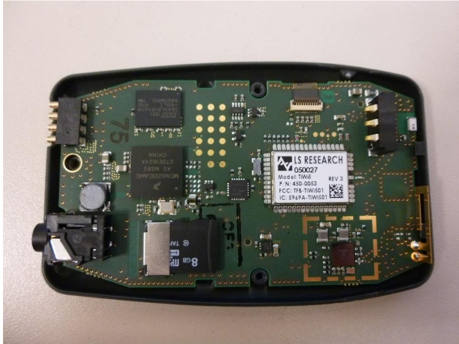
Photo 5: PCB back side view
