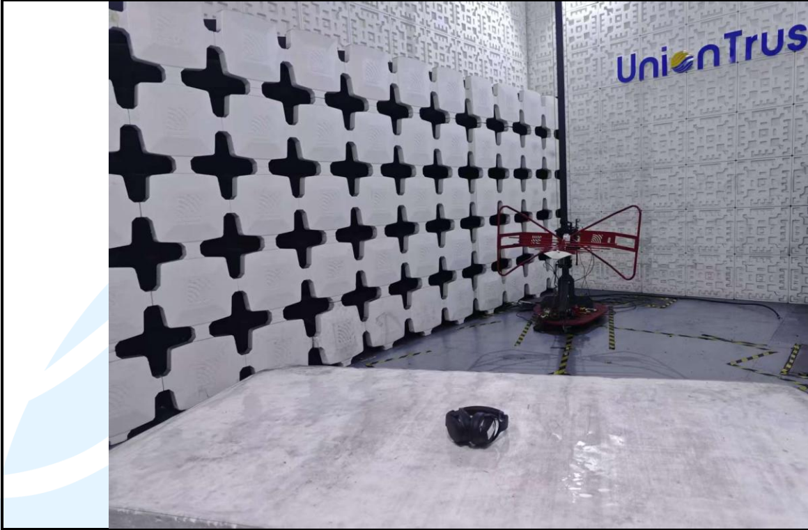
Radiated emission Test Setup (30 MHz~1 GHz)
