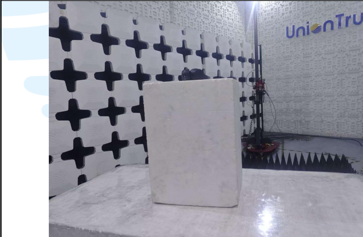
Radiated emission Test Setup (Above 1 GHz)
