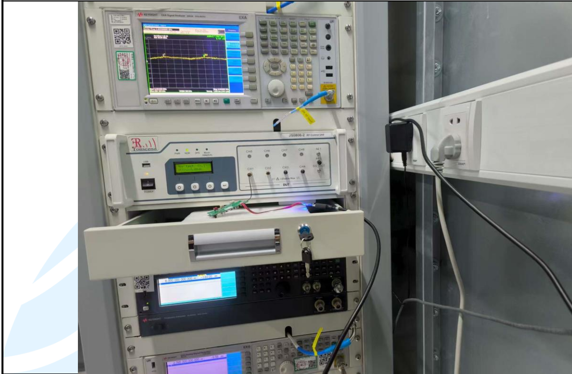
RF Conducted Test Setup
