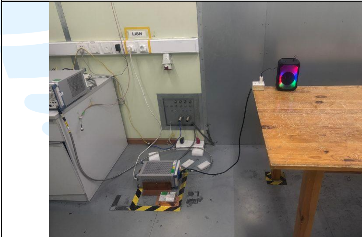
Conducted Emission Test Setup
