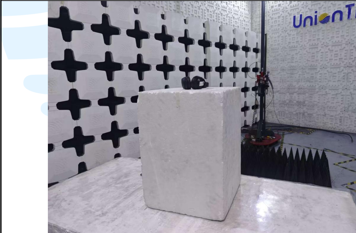
Radiated emission Test Setup (Above 1 GHz)
