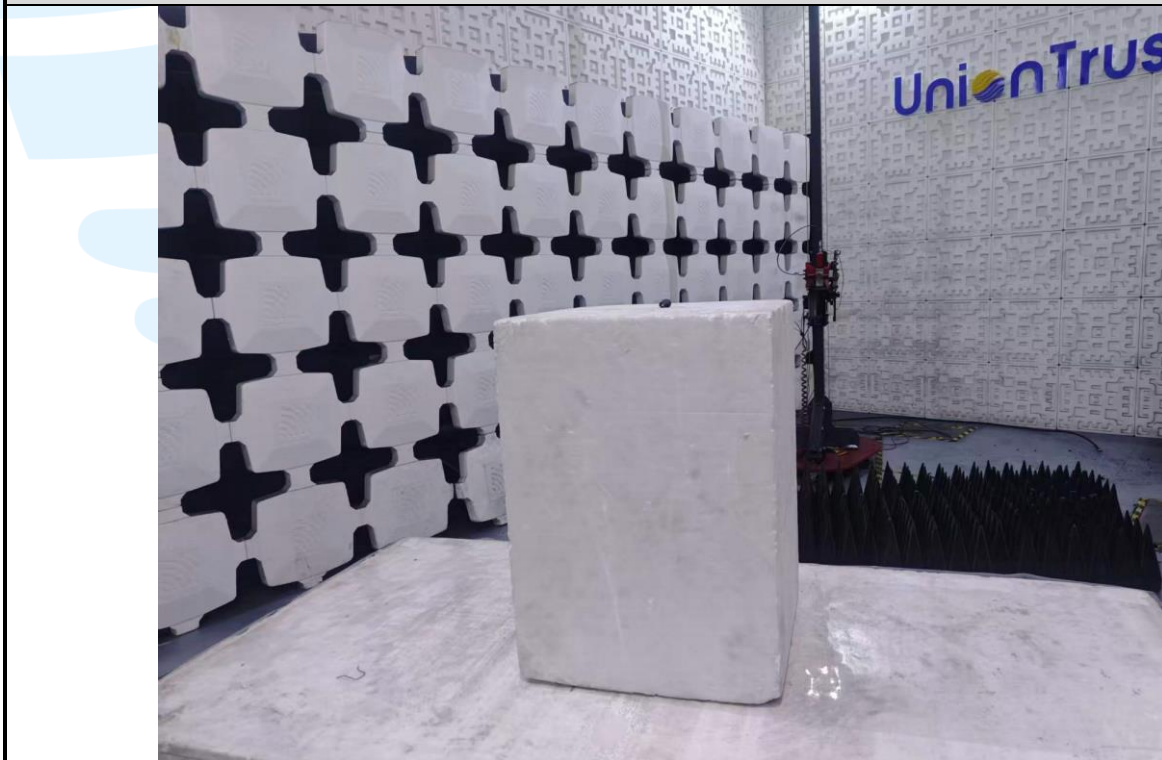
Radiated emission Test Setup (Above 1 GHz)
