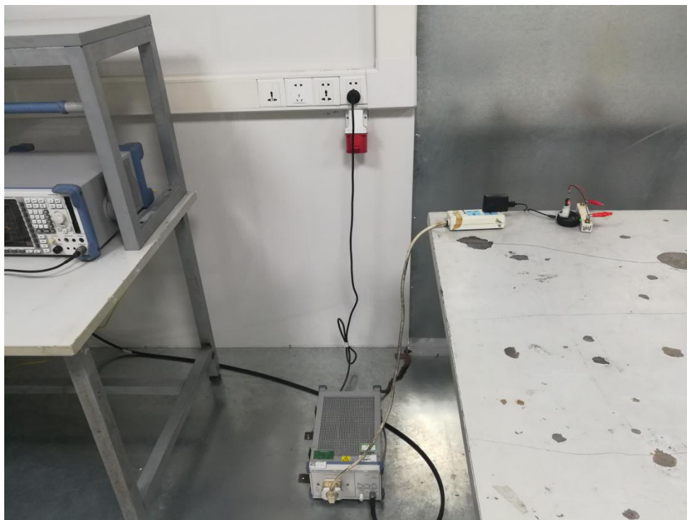
Photo of Conducted Emission Measurement
