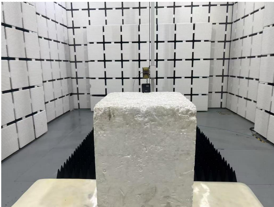
Set-up for Radiated Spurious Emission, Above 1GHz
