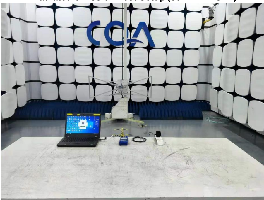
Radiated emission Test Setup (30MHz~1GHz)
