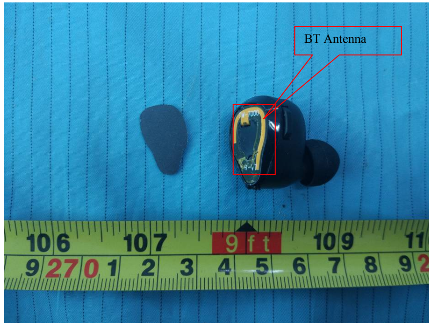
EUT – Cover off View 1
