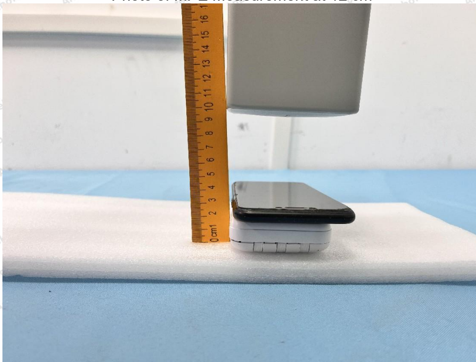
Photo of MPE Measurement at 12 cm
