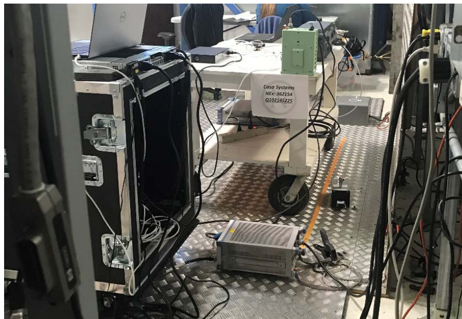
Figure 8.2-4: Conducted disturbance at mains port setup photo
