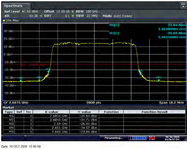
Figure 8.2-44: Conducted band edge emissions for 16QAM 2687.5 MHz, 5 MHz channel - Port 1
