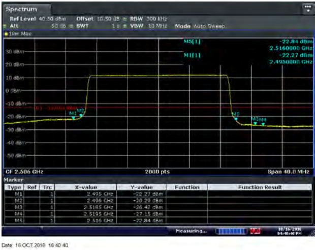
Figure 8.2-55: Conducted band edge emissions for QPSK 2506 MHz, 20 MHz channel - Port 1
