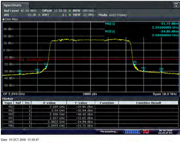
Figure 8.2-41: Conducted band edge emissions for 16QAM 2593 MHz, 5 MHz channel - Port 1
