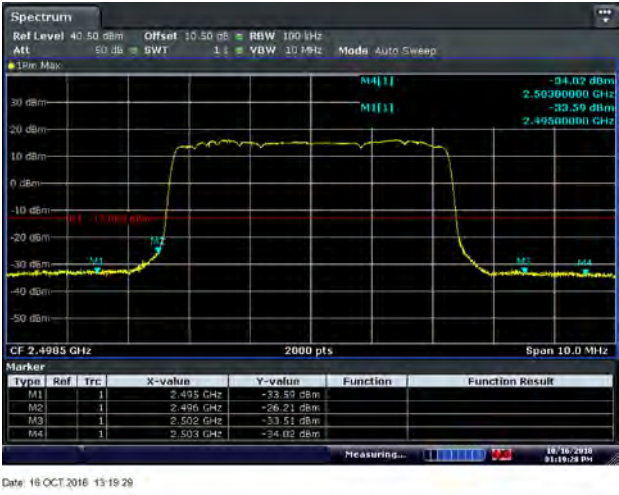
Figure 8.2-36: Conducted band edge emission for 16QAM 2498.5 MHz, 5 MHz channel - Port 1
