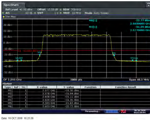
Figure 8.2-59: Conducted band edge emissions for 16QAM 2593 MHz, 20 MHz channel - Port 1
