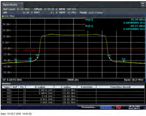
Figure 8.2-45: Conducted band edge emissions for 64QAM 2687.5 MHz, 5 MHz channel - Port 1
