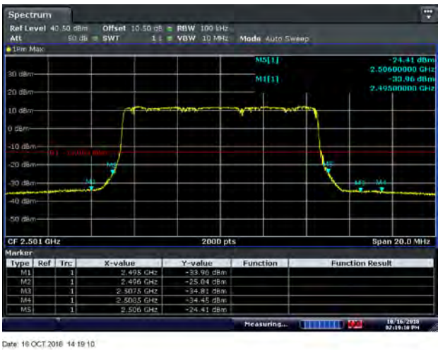
Figure 8.2-47: Conducted band edge emissions for 16QAM 2501 MHz, 10 MHz channel - Port 1
