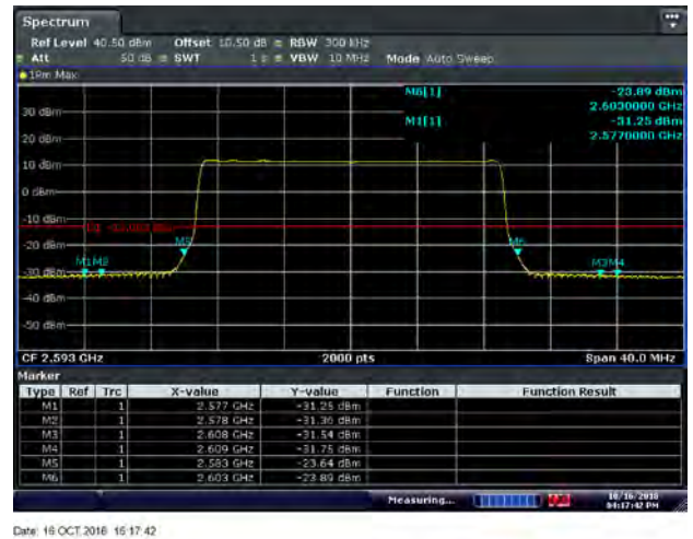
Figure 8.2-58: Conducted band edge emissions for QPSK 2593 MHz, 20 MHz channel - Port 1
