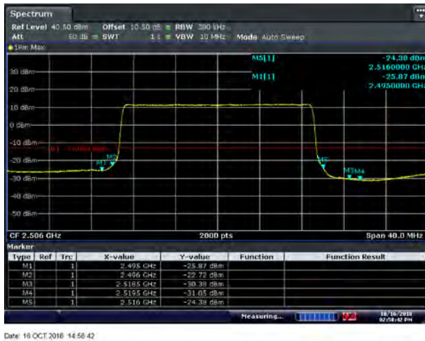
Figure 8.2-57: Conducted band edge emissions for 64QAM 2506 MHz, 20 MHz channel - Port 1
