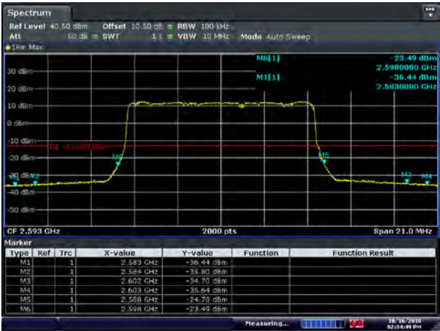
Figure 8.2-50: Conducted band edge emissions for 64QAM 2593 MHz, 10 MHz channel - Port 1
