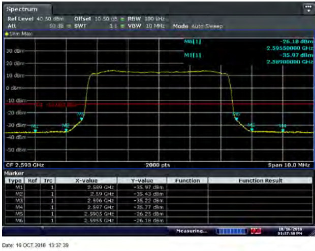
Figure 8.2-42: Conducted band edge emissions for 64QAM 2593 MHz, 5 MHz channel - Port 1
