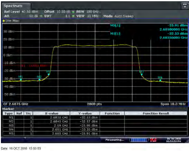
Figure 8.2-43: Conducted band edge emissions for QPSK 2687.5 MHz, 5 MHz channel - Port 1
