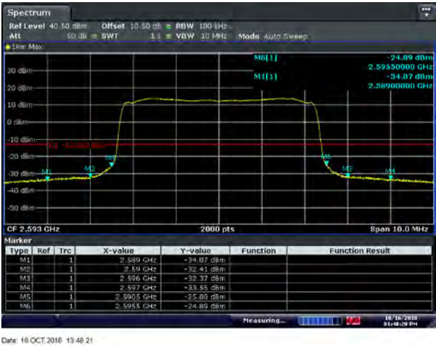
Figure 8.2-40: Conducted band edge emissions for QPSK 2593 MHz, 5 MHz channel - Port 1
