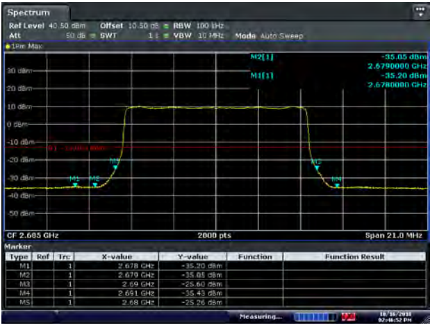
Figure 8.2-52: Conducted band edge emissions for QPSK 2593 MHz, 10 MHz channel - Port 1
