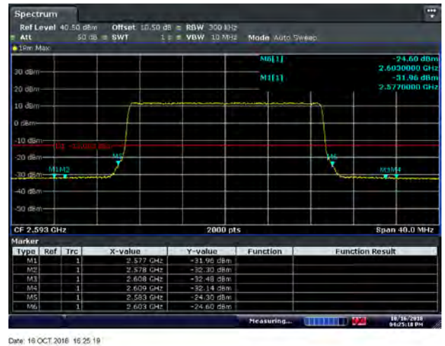
Figure 8.2-60: Conducted band edge emissions for 64QAM 2593 MHz, 20 MHz channel - Port 1
