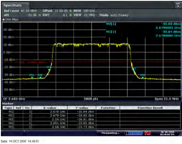
Figure 8.2-53: Conducted band edge emissions for 16QAM 2685 MHz, 10 MHz channel - Port 1
