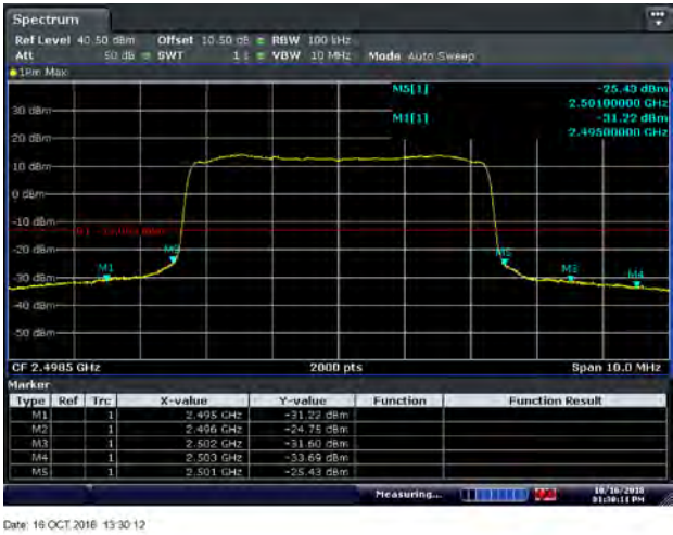
Figure 8.2-39: Conducted band edge emissions for 64QAM 2498.5 MHz, 5 MHz channel - Port 1
