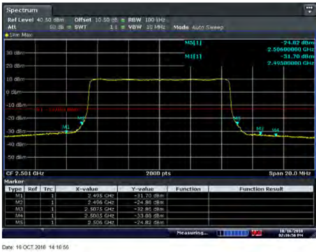
Figure 8.2-46: Conducted band edge emissions for 64QAM 2501 MHz, 10 MHz channel - Port 1
