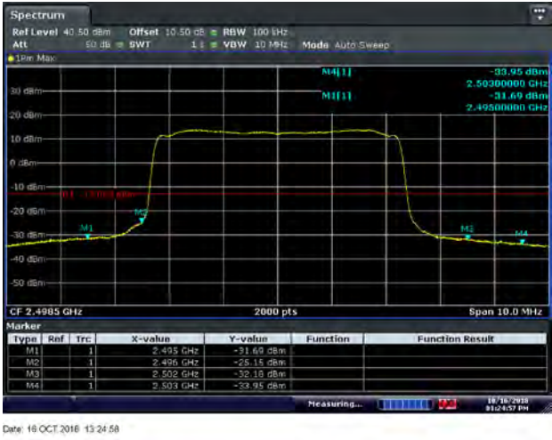
Figure 8.2-37: Conducted band edge emissions for QPSK 2498.5 MHz, 5 MHz channel - Port 1
