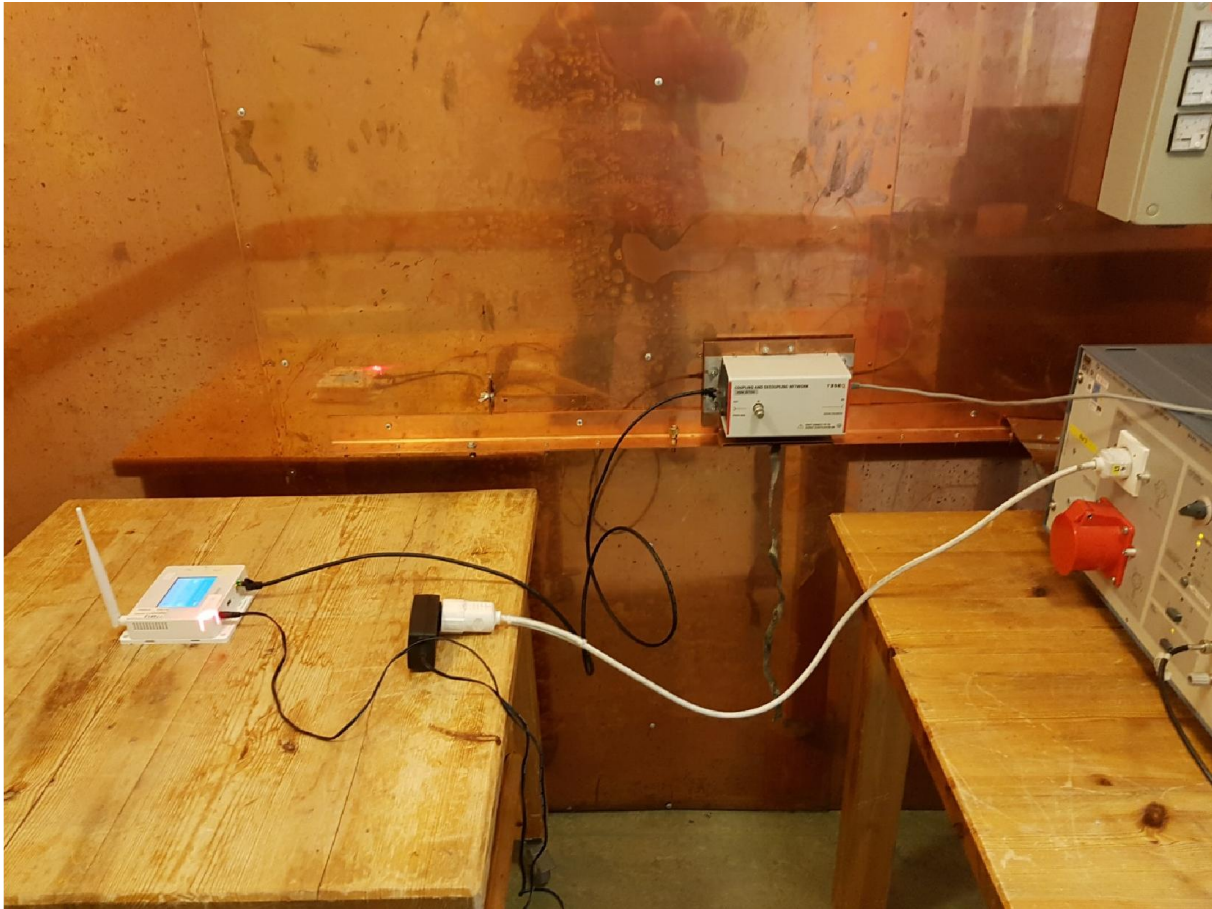
Test set up Conducted emission 150 kHz – 30 MHz
