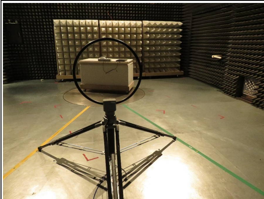
Test setup below 30 MHz - view 2
