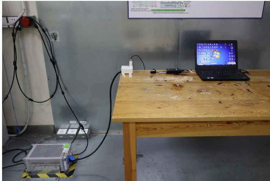
Photograph 3: Set-up for Conducted Emission on AC Mains
