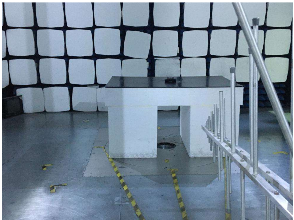
Radiation Emission Test Setup (30 MHz to 1 GHz)
