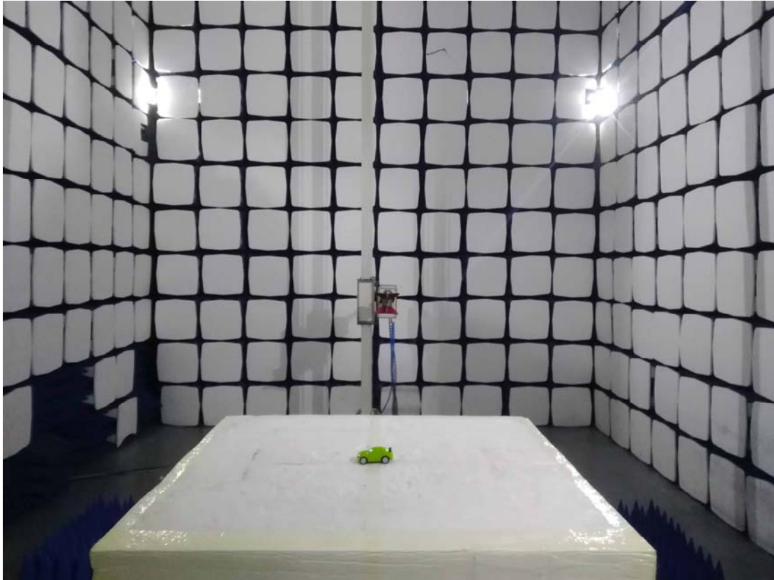
Radiated Emission Test Setup (from 1 GHz to 18 GHz) from 1.5M-Height Turntable Test Table
