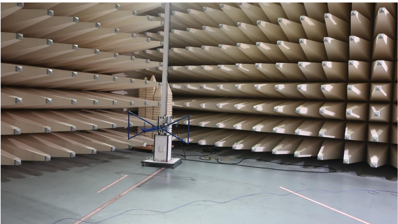
Photograph 4: Setup of radiated emissions measurement in the frequency range 30 – 1000 MHz (rear)
