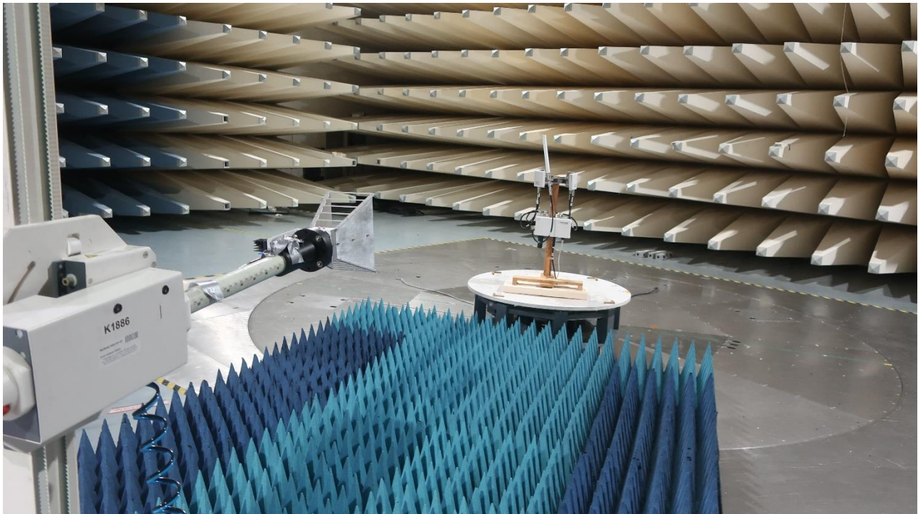
Photograph 5: Setup of radiated emissions measurement in the frequency range over 1 GHz (front)
