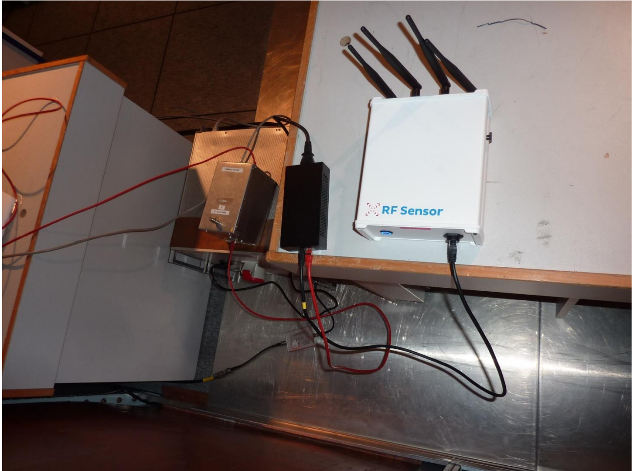
162281_EUT59.: Conducted emissions measurment
