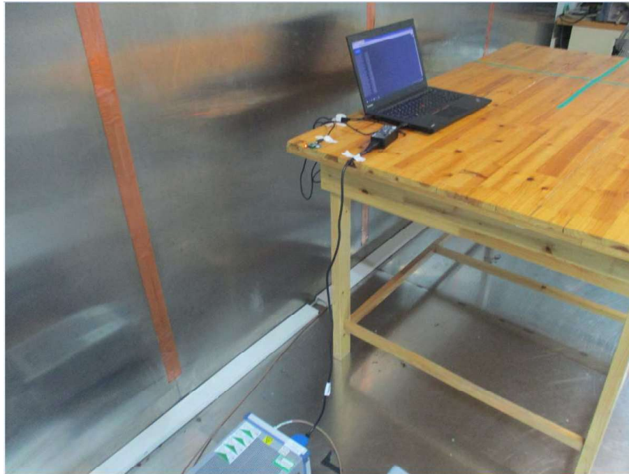
Photograph 1: Set-up for measurement of conducted emission
