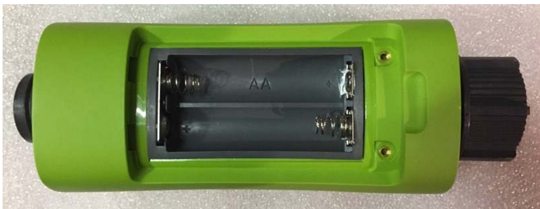
Side 3 with battery cover removed.
