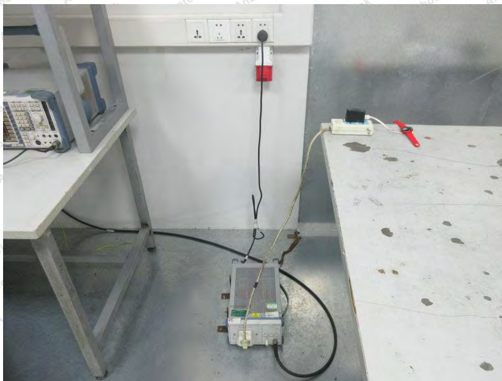
Photo of Power Line Conducted Emission Test
