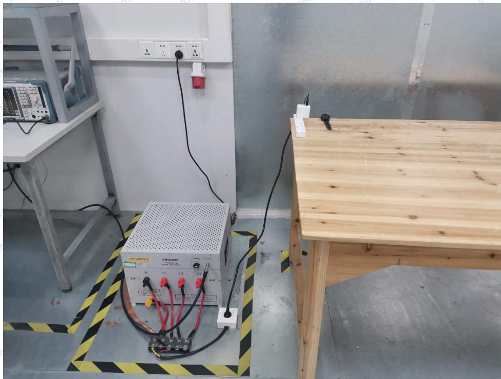
Photo of Conducted Emission Measurement
