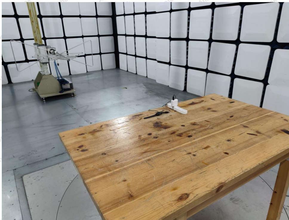
Photo of Radiation Emission Test
