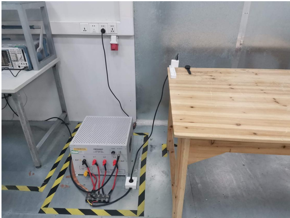
Photo of Conducted Emission Measurement
