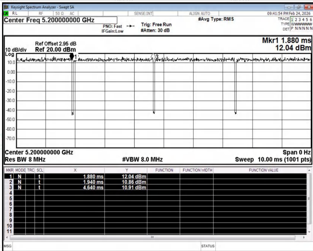
Duty Cycle NVNT a 5200MHz Ant1
