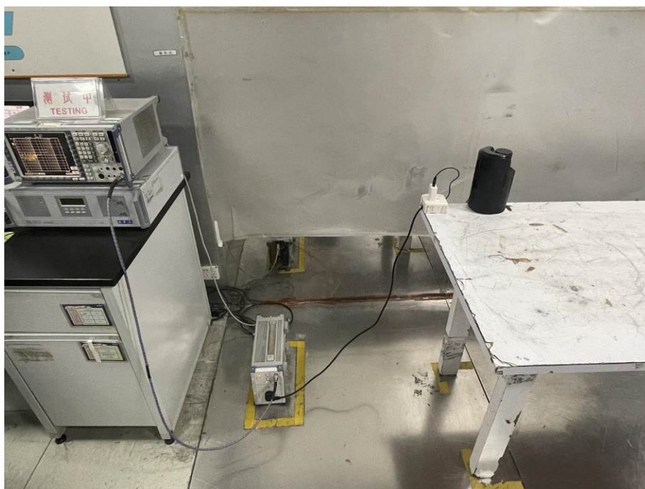
Conducted Emissions Test Setup
